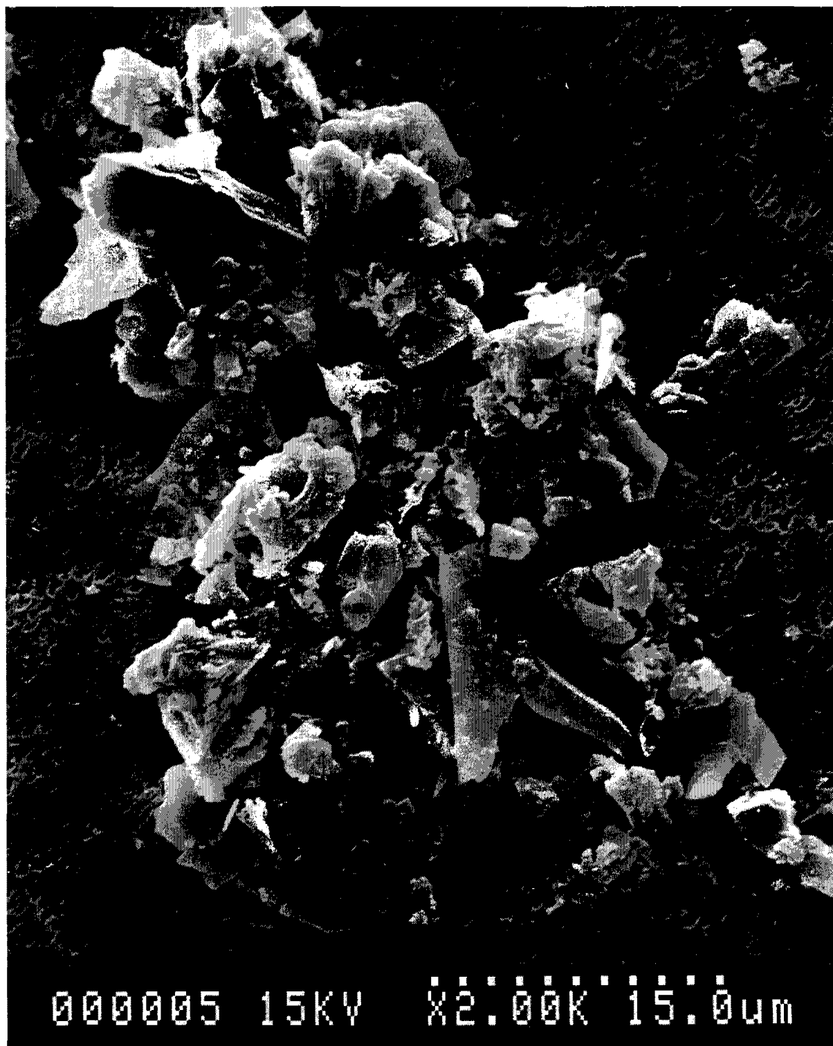
Plate 6.3 Floc as seen under the scanning electron microscope
